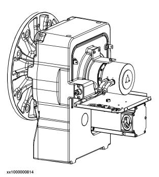
The function is to transfer air/water between a fixed part and a moving part. Technical specification, see table below.
